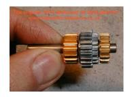
The output shaft fully assembled.
